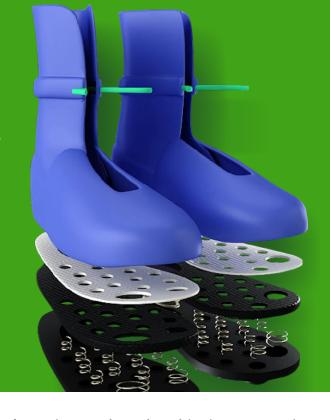
The foot sleeve is a sock and cushioning suspension system that an athlete can wear that goes inside of a shoe (sneaker). The foot sleeve will extend up to the players knees and will have small tensioner springs that flexes and moves with the athlete while running and in motion.
